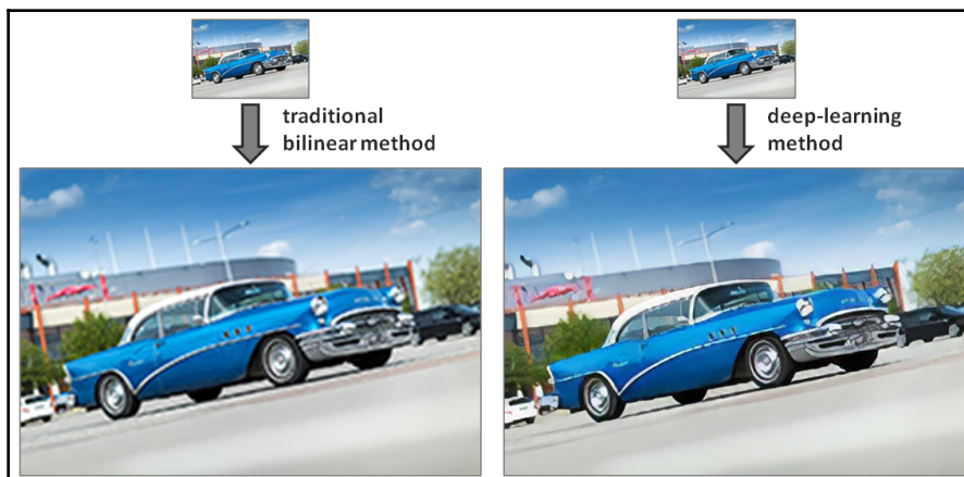
Figure 1.7: Comparison of traditional and deep learning methods for image super-resolution. Notice how the details are sharper in the second image
