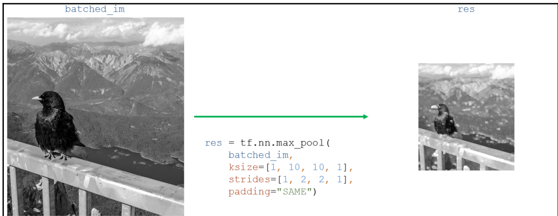
Figure 3.8: Example of another max-pooling operation, with an excessively large window size compared to the stride (purely for demonstration purposes)
