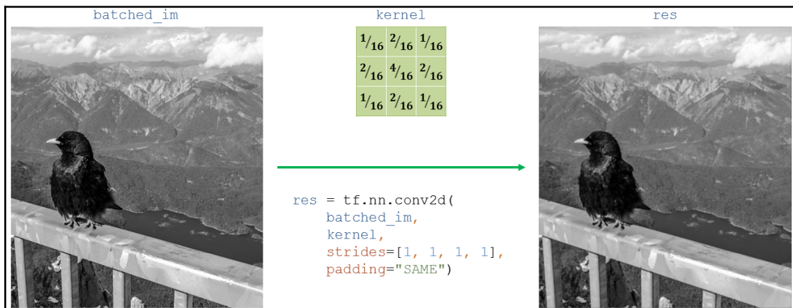
Figure 3.3: Example of a convolution performed on an image with TensorFlow. The kernel here is a well-known one, commonly used to apply Gaussian blur to images
